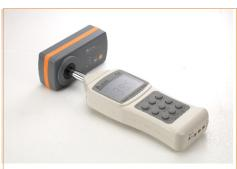
Designed to be used for ANSI S1.40-2006 to calibrate sound level meter with about ½" microphone diameter
